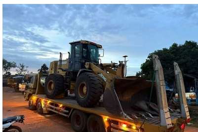
Lowbed truck carrying a wheel loader.
