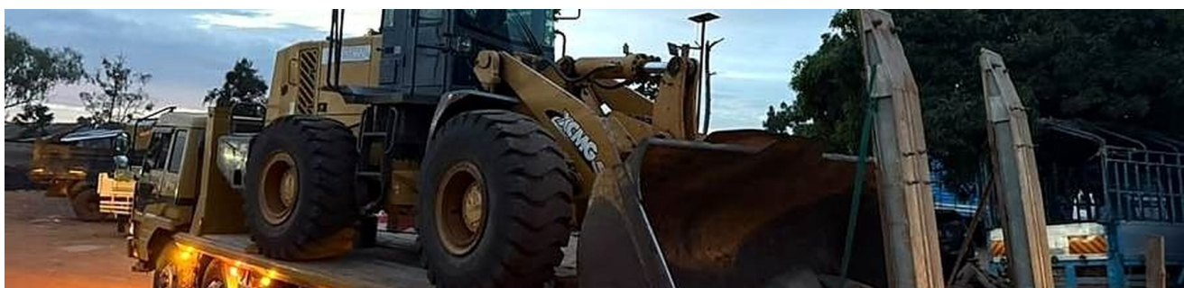
Lowbed trailer carrying a wheel loader to site.
